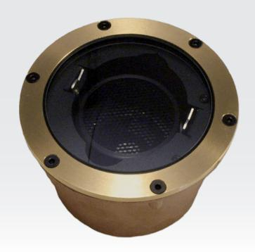
Precision cast and machined LED lighting fixture with 12V input LED Light Engine (COB with integrated driver module). Modular industry standard components allow for simple field replacement and future upgrade. Rugged cast bronze construction is suitable for the most corrosive of environments and is designed for in ground mounted up lighting in wet location landscape applications.
